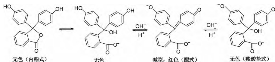
Fig 1 Structural changes of phenolphthalein in alkaline solution
